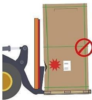
Figure 7 It is forbidden for the raised part of the fork to be in direct contact with the carton
